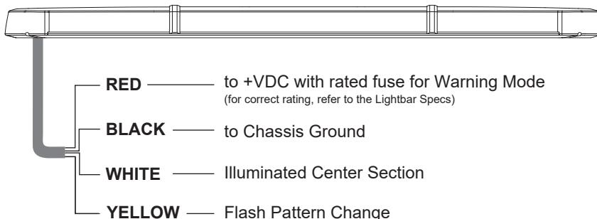
**NOTE:** All function wires (Inputs) are activated by applying +VDC continuously.
